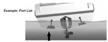
Increase Lift Pressure on port side tab to correct list
