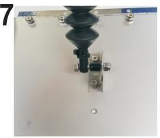
Attach the actuator: Use the hardware from Bag "B" to attach the actuator to the middle hole #3 (medium pressure). Tighten the bolt down just enough so that the actuator can still move freely. Use the black push pin in Bag B to fill the extra hole in the plate if not used.
