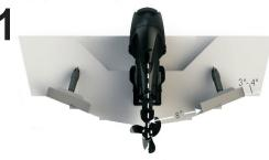
Choose The Location: Preferably inside the chine. You don't want any part of the tab any closer than 8" to the centerline of the boat. Align the bottom of the hinge flush with the bottom of
