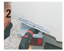
Mark Mounting Holes: Use the hinge template. Make sure that you can mount the hinge in the same location on both sides of the boat. Use a 7/32" drill bit for Fiberglass transoms and a 3/16" drill bit for aluminum and wood transoms.
