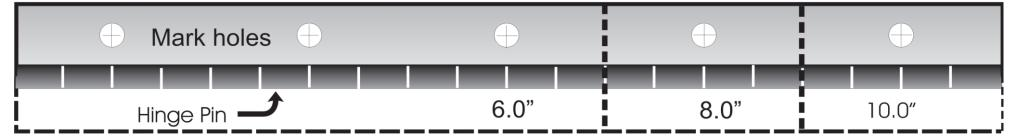
Align dotted line with bottom edge of hull (hinge pin /plate will be 1/2" up from bottom)
