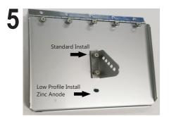
Attach the Plate Bracket: Align the bracket from Bag "B" onto the trim plate using the 2 holes closest to the hinge. The third hole is for a zinc anoide or if you have height clearance issues you can move the bracket to these holes and this will give you 2.5" less height clearance.
